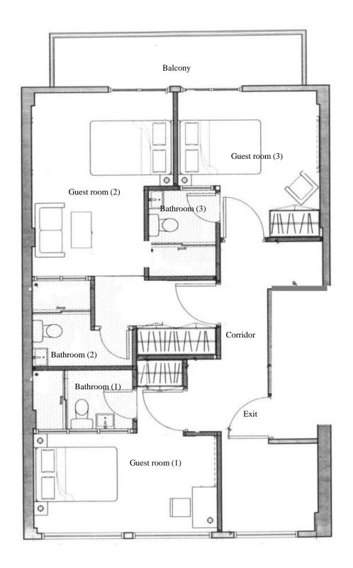
$\S$  The plan is only for illustration of the typical layout of holiday flat of guesthouse layout. Applicant may refer to Chapter II for the building safety conditions and Chapter III for the fire safety conditions respectively. Upon submission of application and the proposed holiday flat layout, the Office of the Licensing Authority will formulate detailed upgrading requirements and notify the applicant accordingly.
